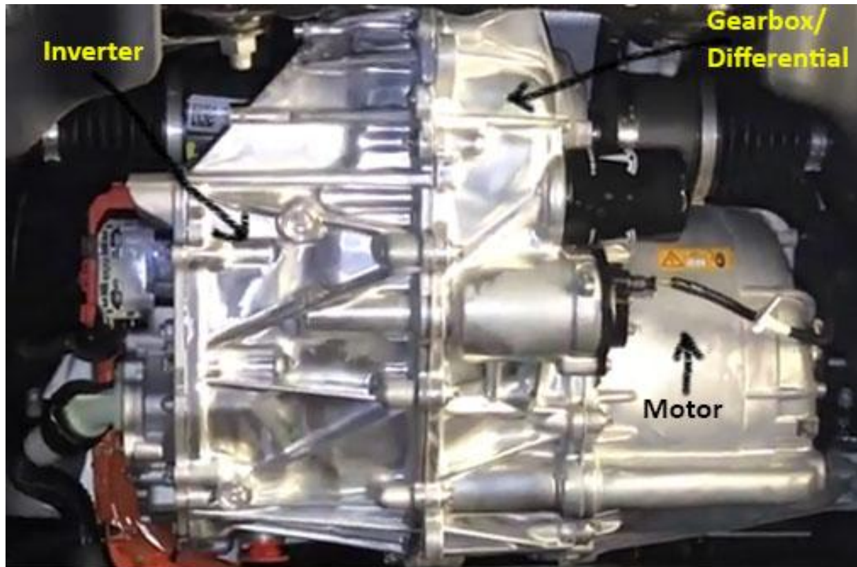
Photo of Model 3 motor from underneath car. Courtesy of EVTU.
